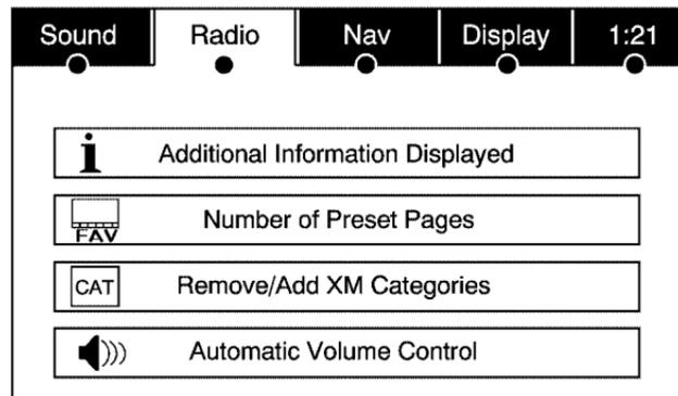
Press the MENU key to enter the menu screen, then press the MENU key repeatedly until Radio is selected or touch the Radio screen button to make changes for radio information displayed, number of preset pages, XM categories, and Automatic Volume Control or Bose® AudioPilot®.
