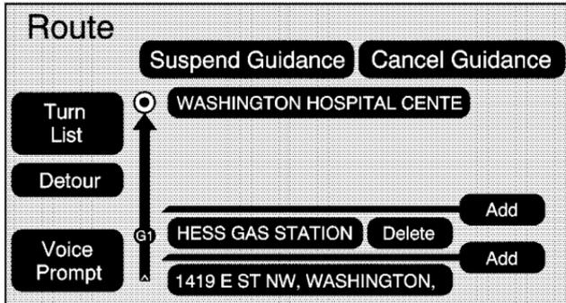
**Add Waypoint:** Select this screen button from the Route screen. This feature allows you to add up to three waypoints to the current route, between your start point and final destination. Once a waypoint has been added, the points can be edited or deleted.
