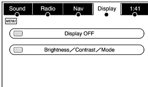
Press the MENU key to enter the menu options, then press the MENU key repeatedly until Display is selected or touch the Display screen button.
