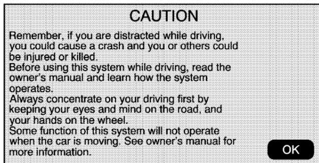
Each time the vehicle is started and the navigation system is turned on, the Caution screen or the previous active screen will appear dependent on system power off time. If the Caution screen appears, touch OK to load the map DVD information. If OK is not selected, all hard keys except for NAV (navigation) and DEST (destination) can be accessed. Once the NAV or DEST hard keys are pressed, this Caution screen will appear and OK must be pressed to load the map DVD information from the map disc.
