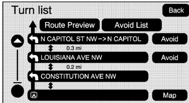
**▲/▼ (Scroll Arrows):** Touch the up and down arrow screen buttons to scroll through the list of maneuvers.
