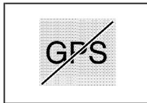
The No GPS symbol will appear when your vehicle is not receiving a Global Positioning System (GPS) satellite signal.
