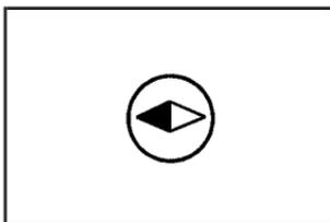
The heading up symbol indicates the map with the vehicle travel direction up, known as Heading Up mode.
